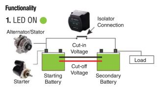
1. When the voltage of the starting battery reaches 13.3V, the isolator is engaged. The two batteries charge simultaneously. The LED indicator will be on.
