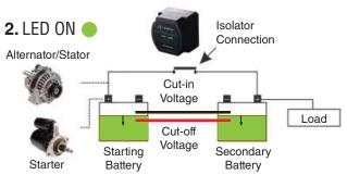
2. When the batteries are no longer being charged by the alternator, and both batteries are being drained. The LED indicator will be on.
