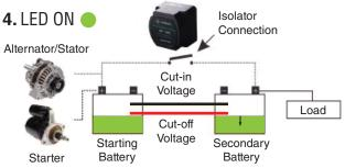
4. When the vehicle is restarted and the starting battery reaches 13.3V, the isolator will reengage. The LED indicator will be on.
