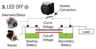
3. When the voltage drops below 12.8V for 5 seconds, the isolator senses this and disengages, separating the batteries. The LED indicator will be off.
